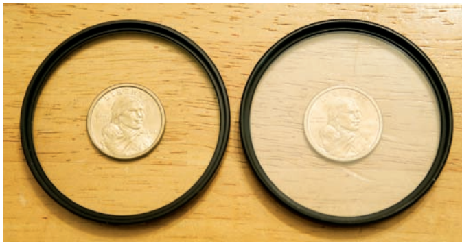
Figure 2.46: Use a multicoated filter (left) for maximum light transmission
