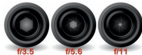
Figure 2.25: A lens aperture is an adjustable hole that controls how much light comes into the camera
