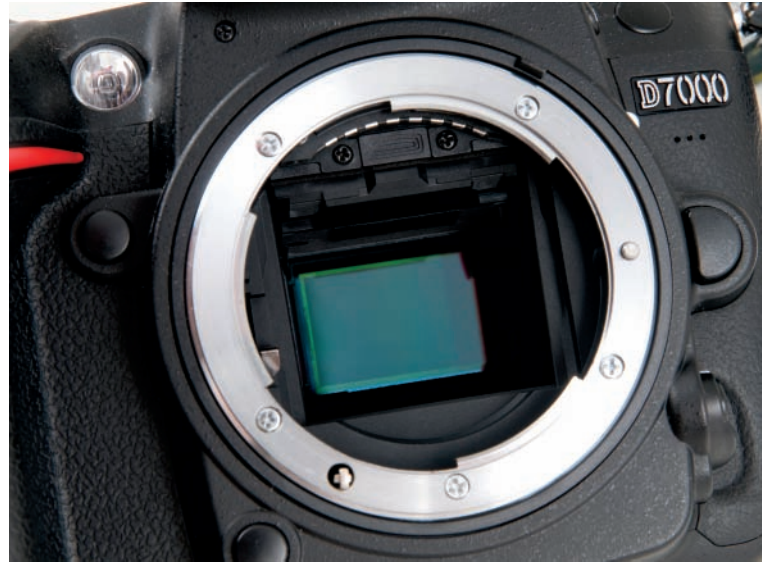
Figure 1.5: The imaging sensor inside a Nikon DSLR, as seen with the lens removed. The reflex mirror was raised in this picture to expose the sensor.
