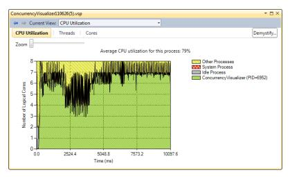
In the preceding graphic, the y-axis represents the logical cores, and the x-axis is the timeline, shown in milliseconds. There is a Zoom slider control above the graph. Drag right to enlarge the graph. You can also drag the mouse horizontally across the graph to zoom in to a portion of the graph.
