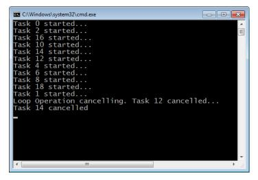
And the next image shows some output from the end of that same application. Notice that tasks with an index value less than 12 were allowed to start or run to completion.
