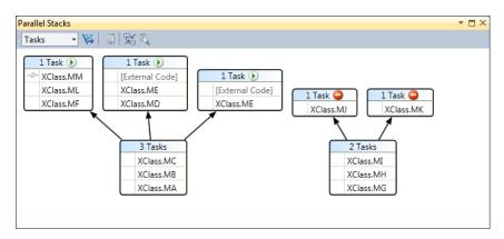
The preceding diagram shows five tasks. Two threads execute on the same call stack, which is {*MI*, *MH*, *MG*}. One of the tasks then calls *MJ*. The other task calls *MK*. Three threads share the {*MC*, *MB*, *MA*} call stack before separating paths. If you point to a node header, you will display a tooltip with information on each task in the call stack. If you point to the header with three tasks, here's what is displayed:
