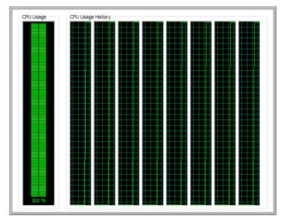
You'll delve into the syntactical nuances of *Parallel.For* shortly. The important point now is that this code successfully parallelizes the operation as a basket of tasks scheduled across the available cores. There are enough tasks to keep the processor cores busy, which is an important goal of parallel programming.
