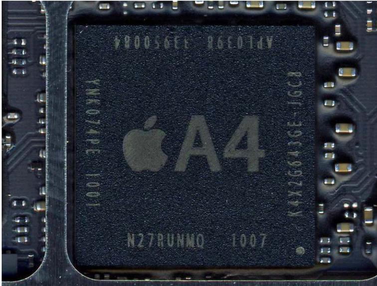
**Figure 3-1.** Apple's proprietary A4 processor
