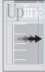
The specs for this page are: 33 × 51 picas, facing pages. The inside margin (in picas) is 3p; outside, 7p; top, 5p; and bottom, 5p. Zero rulers at top center. On the master pages or template, place vertical ruler guides at 29.5, 15.25 and 13.75 picas, both sides of center. Place the horizontal ruler guides at 2, 7 and 47.5 picas. **Note:** The cover has backward margins. Build it to fit a left-hand page, then make it page 1.
