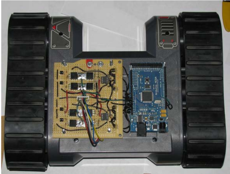
Figure 5-13. The frame base with motor-controller and Arduino mounted
