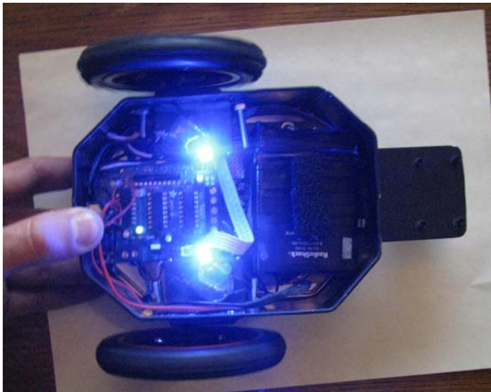
Figure 4-38. Both blue LEDs lit up as the bot is driving forward with both motors
