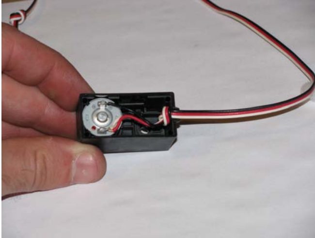
Figure 4-19. Solder the red and white wires to the motor terminal with the red dot beside it, and the black wire to the other terminal. Now it is ready to be re-assembled.
