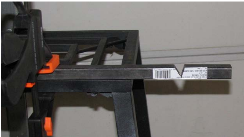
Figure 12-26. Cutting V notches in the weapon brackets
