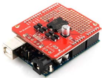
Figure 3-20. The Sparkfun Ardumoto is a motor-controller shield that is built around the L298N dual H-bridge IC.
