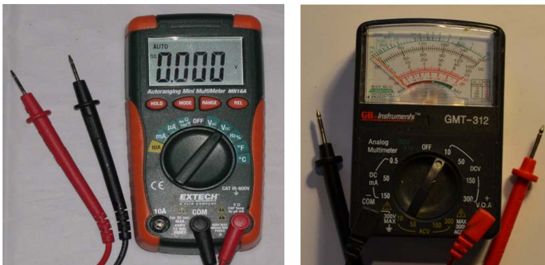
Figure 1-5. The Extech MN16a digital multi-meter (left) measures AC and DC voltages, resistance, continuity, diode test, capacitance, frequency, temperature, and up to 10 amps of current. An inexpensive analog multi-meter purchased at my local hardware store (right) measures DC and AC voltages, resistance (1k ohm), and up to 150mA (0.15A) of current. Either work to diagnose an Arduino and most other circuits—but you definitely need one.
