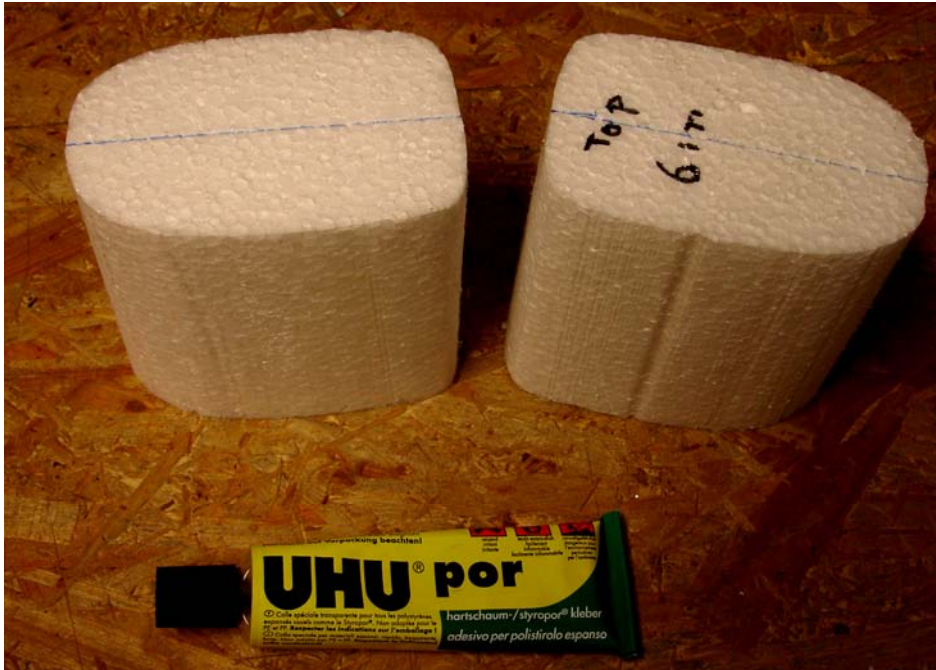
Figure 9-13. Two adjacent segments with EPS/XPS glue
