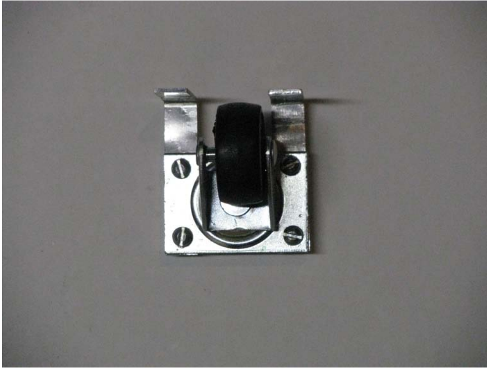
Figure 4-25. The caster wheel with all four bolts secured to the mounting bracket.
