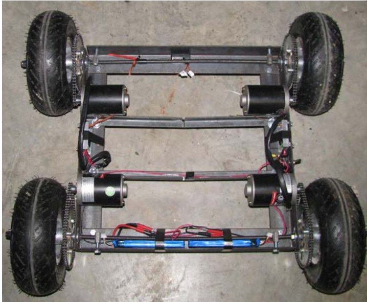
Figure 12-6. The basic frame with motors, wheels, and batteries test-fitted
