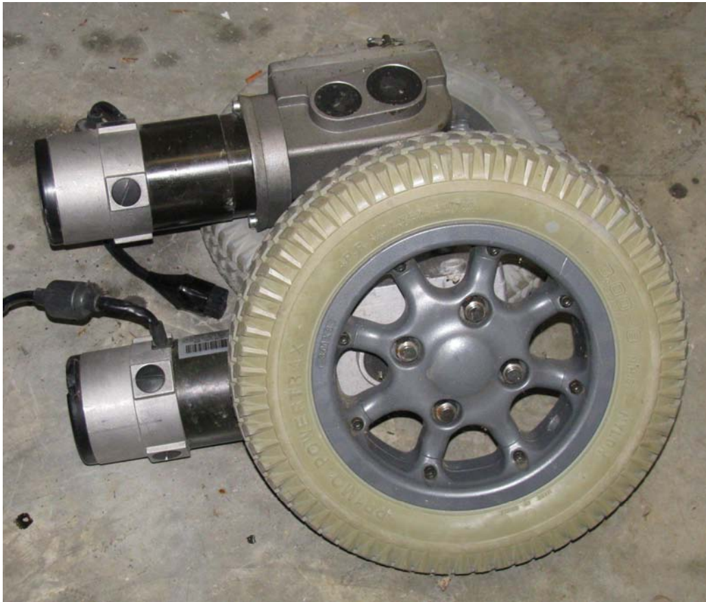
Figure 11-8. The DC gear motors used for the Seg-bot
