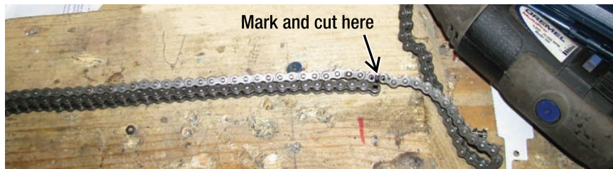
Figure 12-17. Measuring and cutting the chains
