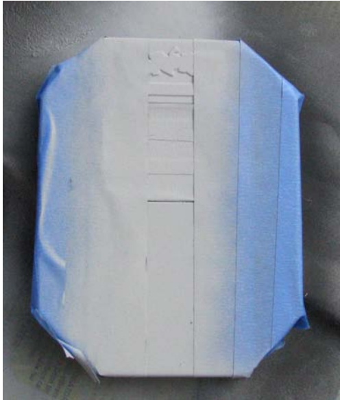
Figure 4-43. Priming the stripe on the lid
