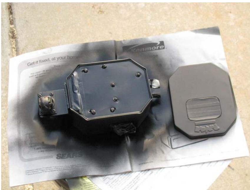
Figure 4-42. The first coat of flat black paint, after the gray primer
