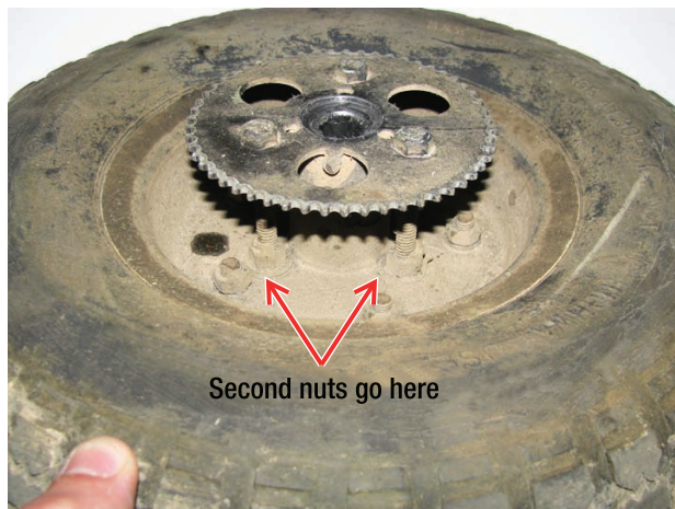
Figure 10-5. The rear wheel with sprocket installed
