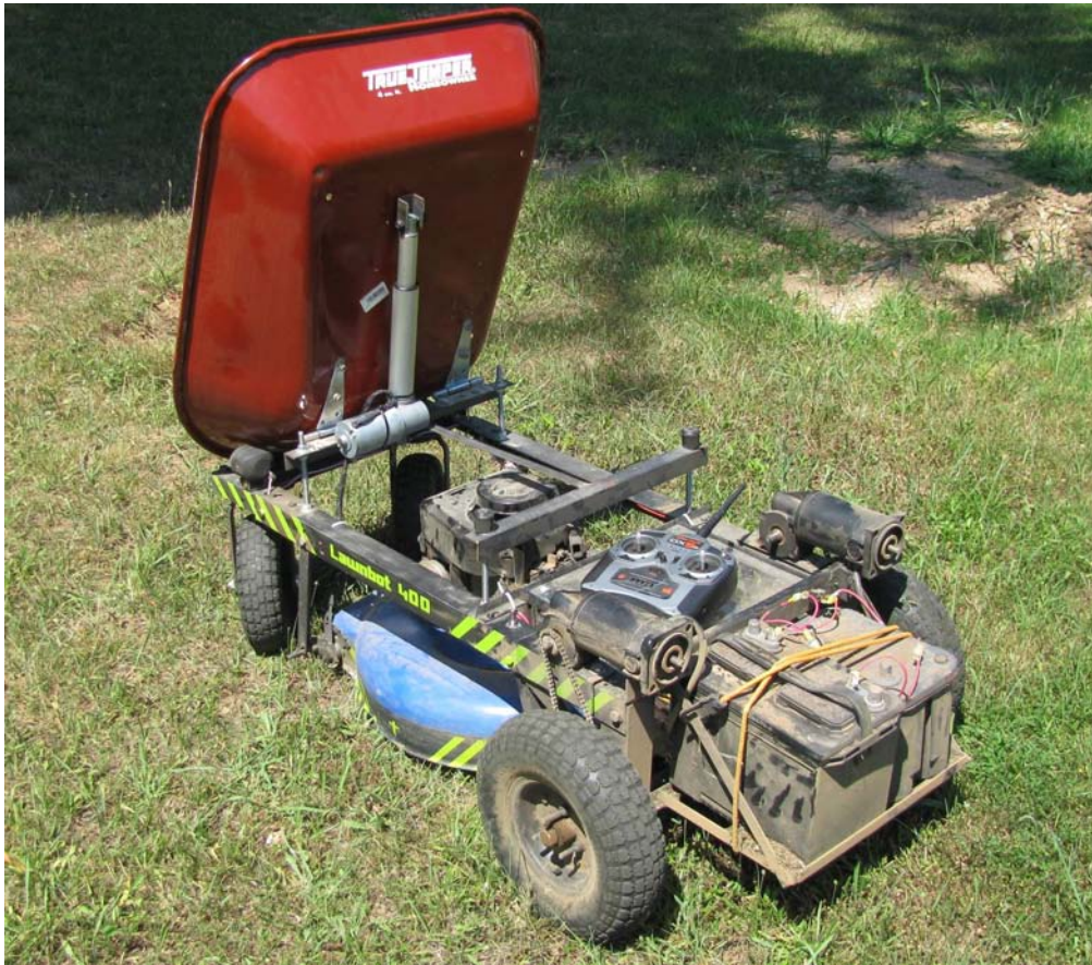
Figure 10-31. The Lawn-bot with dump bucket and linear actuator lift motor installed
