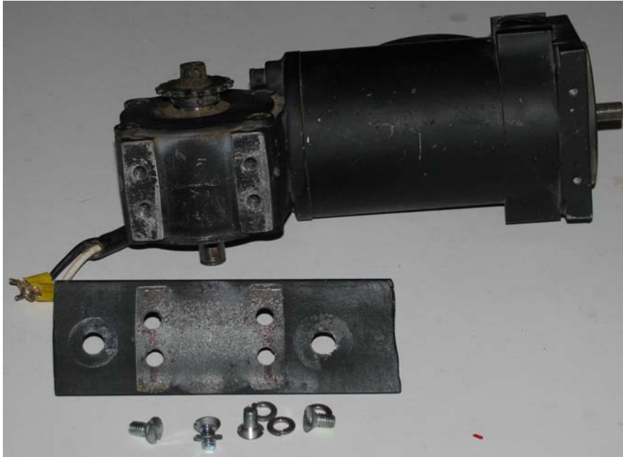
Figure 10-13. The motor mounting plate with 1/4-inch bolts
